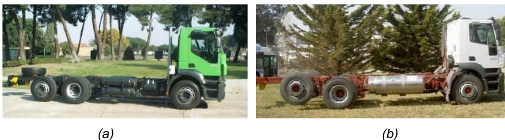
Fig. 3 (a) Comparison CNG vs (b) LNG tank configuration on the same truck chassis
