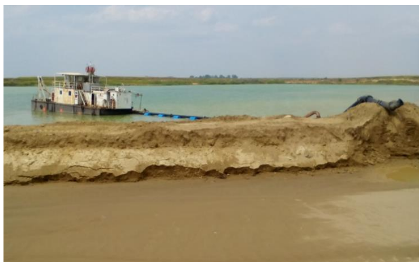
Figure 2: Underwater exploitation system on the surface mine Jakovačka kumša, float suction dredger – pipeline – precipitator
